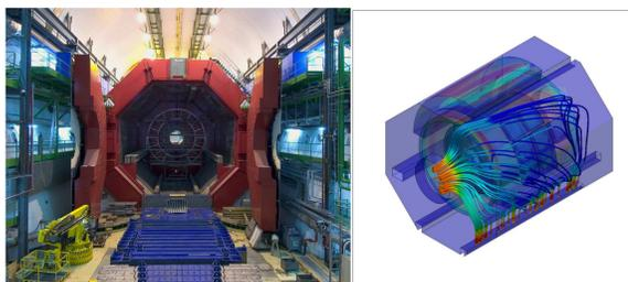
**Problem:** The L3 magnet is a large volume enclosing a number of heat dissipating devices. To achieve optimal particle measurements, the air temperature inside the magnet must be uniform and within a specified limit.
